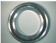
Photo. 6.1 Filling grease into angular contact ball bearing
